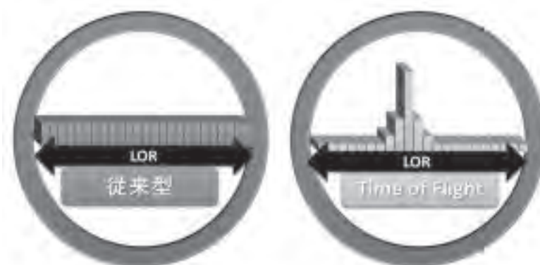
図2 Time of Flight の概念
